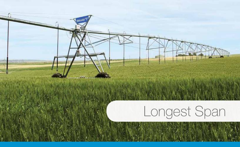
Valmont Irrigation brings you the longest irrigation span in the mechanized irrigation industry reaching up to 72 meters (236'). Currently, the most popular span length is 54.6 meters (180'). The Valley 72-meter span is engineered to the same standards as all Valley Model 8120 spans and has passed the most demanding strength and accelerated life tests in the industry.
